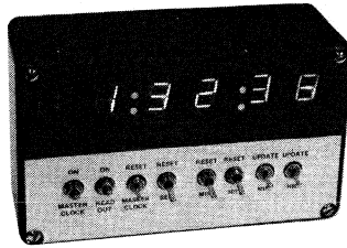
Fig.190 - Photograph of a battery-powered digital Clock that uses Digivac display devices.
